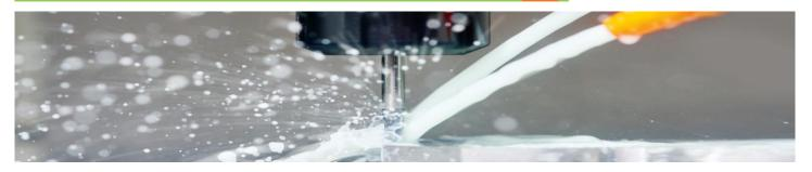
**BANGCHAK CUTTING FLUID CB** is a premium quality, phenol/nitrite free general purpose soluble oil. Forms a milky emulsion to cover the widest range of metal working operations. It offers the following advantages:
