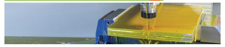
**BANGCHAK NEAT CUT** is a transparent non-corrosive cutting fluid. It is manufactured from paraffinic base oils and contains a chlorinated extreme pressure additive , rust and oxidation inhibitors and a mist-suppressing additive.
